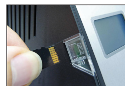
Parameterization thru Micro SD card for of the i-CON Nano
