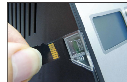
Parameterization thru Micro SD card for of the i-CON pico
